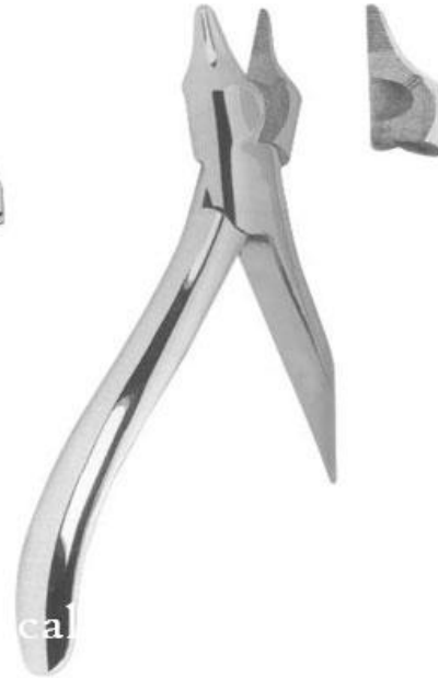
3214 Nance Universal pliers for bending wires up to 0.9 mm. (.035") or cutting up to 0.7 mm. (.028").
