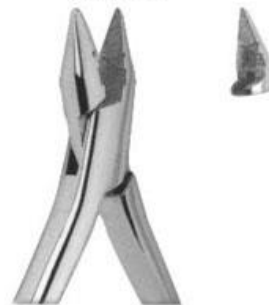
3216 Universal Universal pin roughening, cutting and bending pliers. For wires up to 0.9 mm. (.035"). Will cut wires up to 0.7 mm. (.028").
